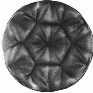
FIGURE 16. A central hexagon (coming from a preimposed smaller one) during Bénard–Marangoni convection in a cylindrical container of 13.5 cm in diameter (courtesy of P. Cerisier).
